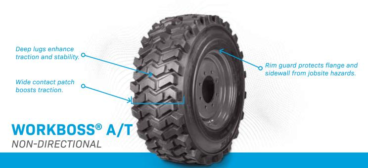
WORKBOSS® A/T with a non-directional tread is a versatile, heavy-duty solution for tough environments. Deep lugs provide added all-terrain traction and stability, especially on uneven surfaces, and promote top self-cleaning performance in muddy conditions. Sidewalls are reinforced and rim guards are included for maximum protection.
